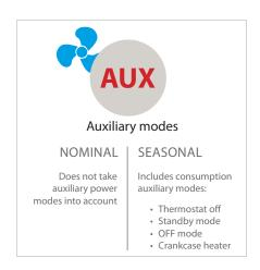
Nominal efficiency gives an indication on how efficient an air conditioner is when operating in a nominal condition.
