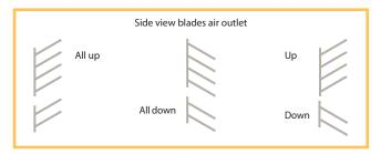
Selectable horizontal out blow to better suit the lay-out of the room (only if connected to BRC1E52A).
